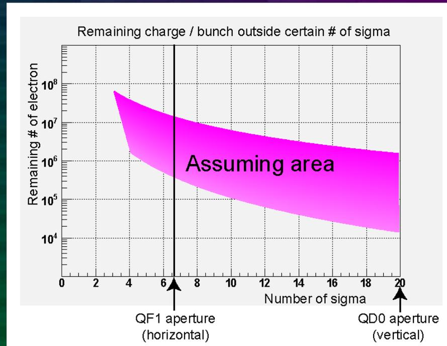
$10^{5\sim 7}$  particles remain outside QF1 aperture ( $6.6\sigma$ )
