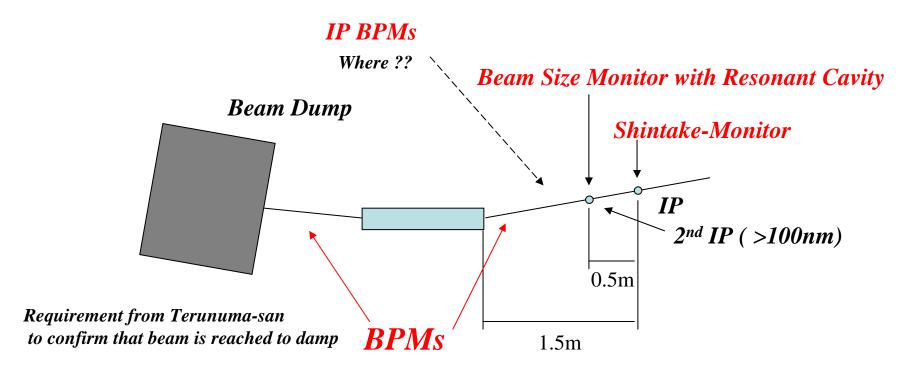
Cavity or Strip-line BPM?? (Beam size is around 2-3mm.)
