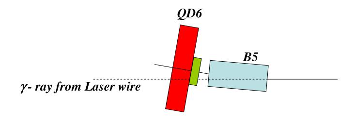
As discussed in  $1^{st}$  ATF2 project meeting in SLAC, we cannot put the C-band cavity BPMs on QD6 to avoid the  $\gamma$ -ray from laser wires.
