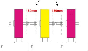
The collimator should be put around SF6 and SF5 for the requirement from the Shintake monitor detector background.
