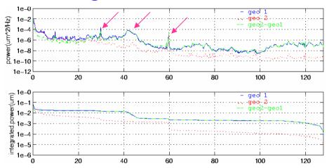
Noise peaks: 60Hz, 30Hz. Broad resonance near 45 Hz. At 3 Hz, the difference is 16nm.
