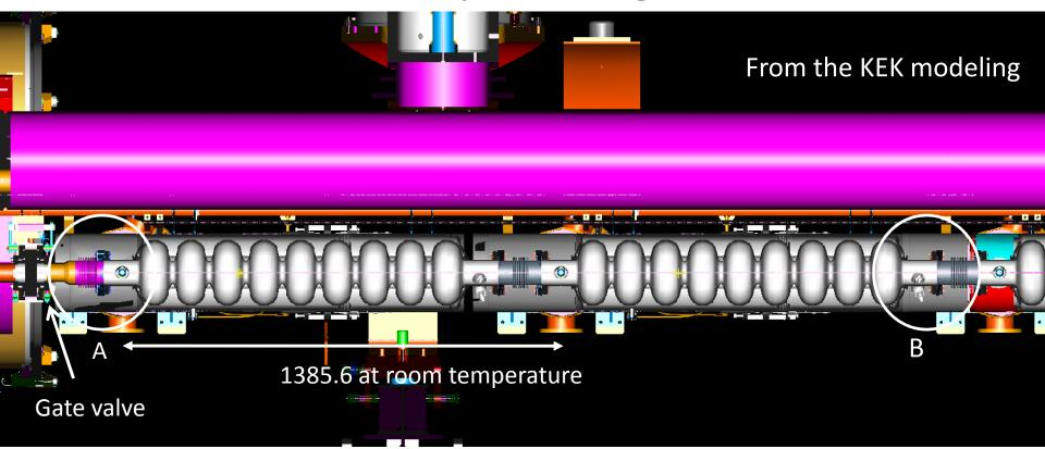
A: The present shield design by FNAL/Don has an interference with the gate valve. The length of the shield in the solid model by Don is 351.5 mm while the length might be 286.5mm.
