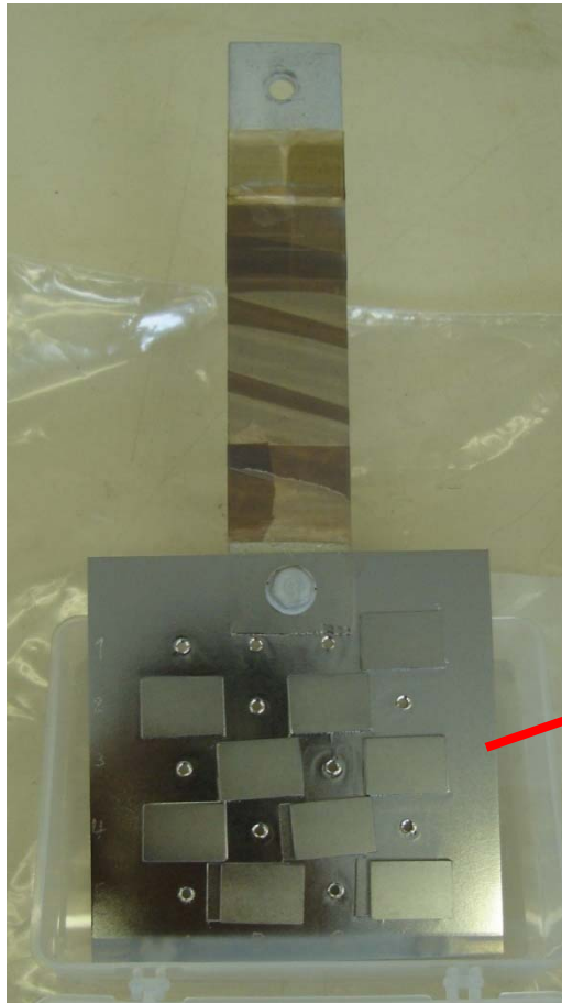
9 square-type Nb samples (10 \mu\text{m} BCP before labo-EP)
