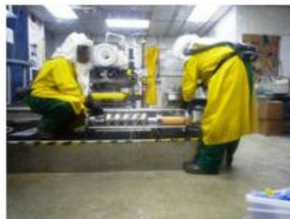
Disassembly of setup and water washing/rinsing
