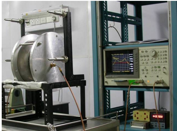
Measure the frequency and coupling factor ( k ) for the dumb-bell
