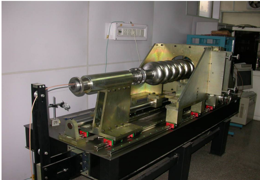
SRF cavity tuning facility
