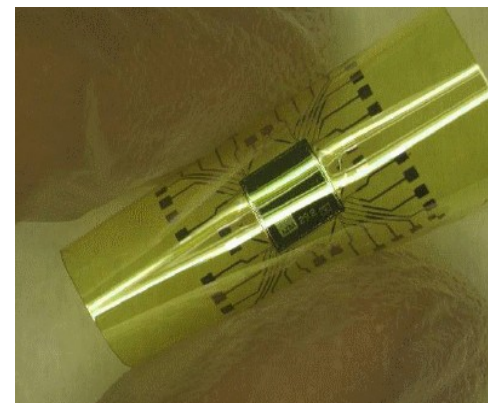
Fully functional microprocessor chip in flexible plastic envelope. Courtesy of Piet De Moor, IMEC company , Belgium
