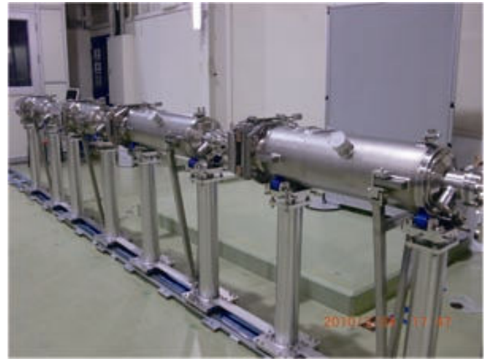
Tuner installation for KEK cavities at outside of clean room
