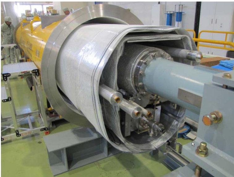
Inserting the cold mass into the vacuum vessel
