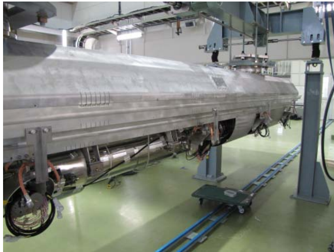
Assembling 5K shield
