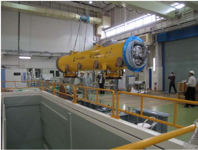
Moving the Module-C into the STF tunnel
