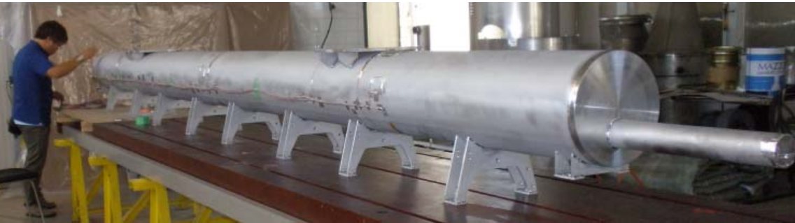
Helium gas return pipe
