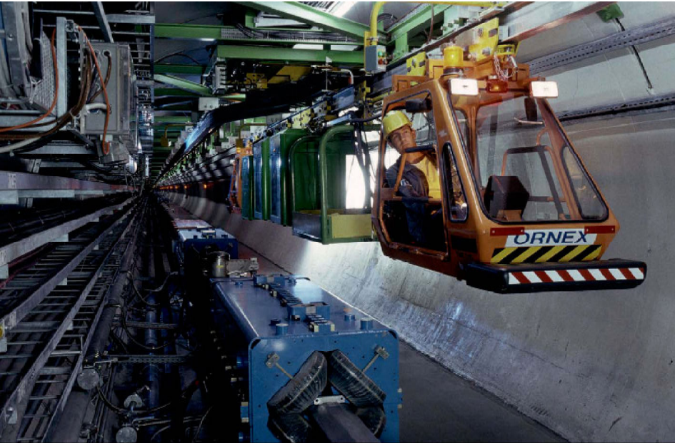
fig.3. translation, alignement, positionnement. TRANSLATION, ALIGNMENT, SETTING.
