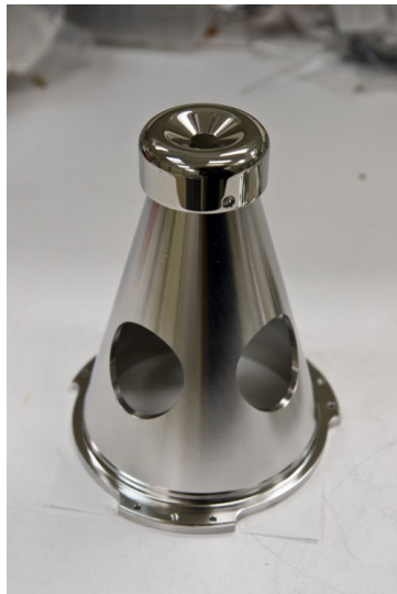
Conventional geometry: cathode electrode mounted on metal support structure
