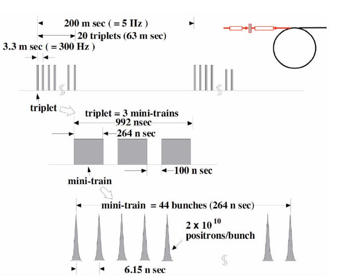
different triplet hit different position on the target
