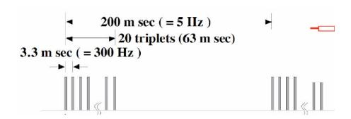
duration of a triplet ~ dumping time of shock wave shoter than time scale of thermal dissusion
