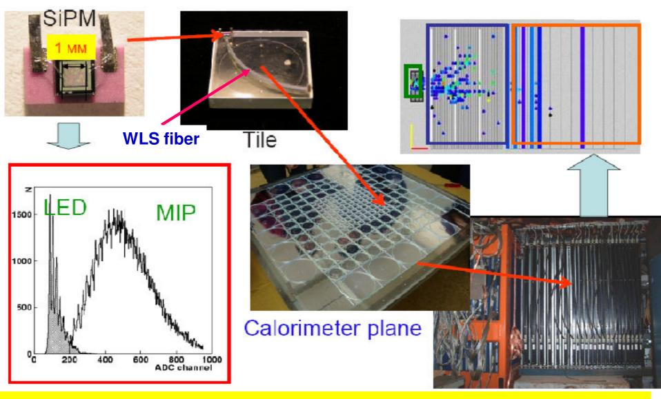
AHCAL with novel SiPM readout demonstrated very reliable performance during beam tests at CERN and FNAL in 2007-2009.
