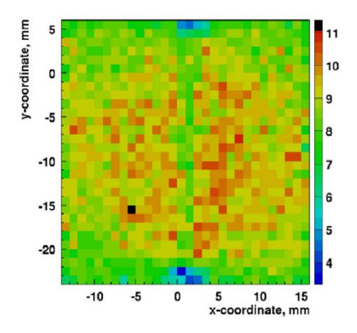
Total efficiency at 0.4 MIP threshold is about 96%
