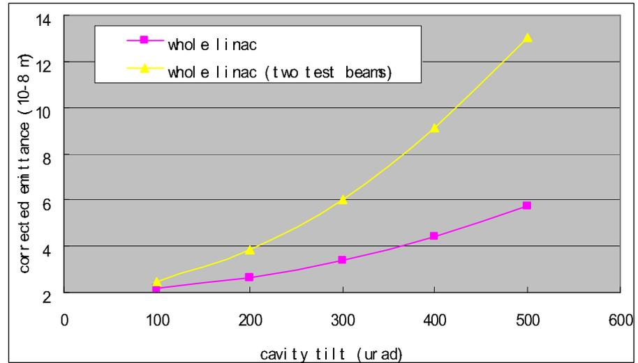
Cavity tilt can not be cured by DFS!
