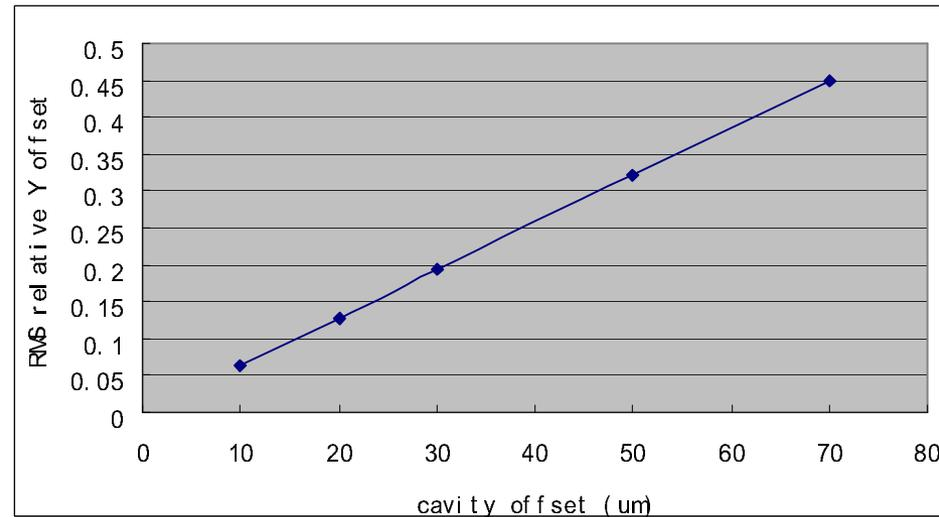
Random cavity position jitter tolerance (about 3% luminosity reduction):
