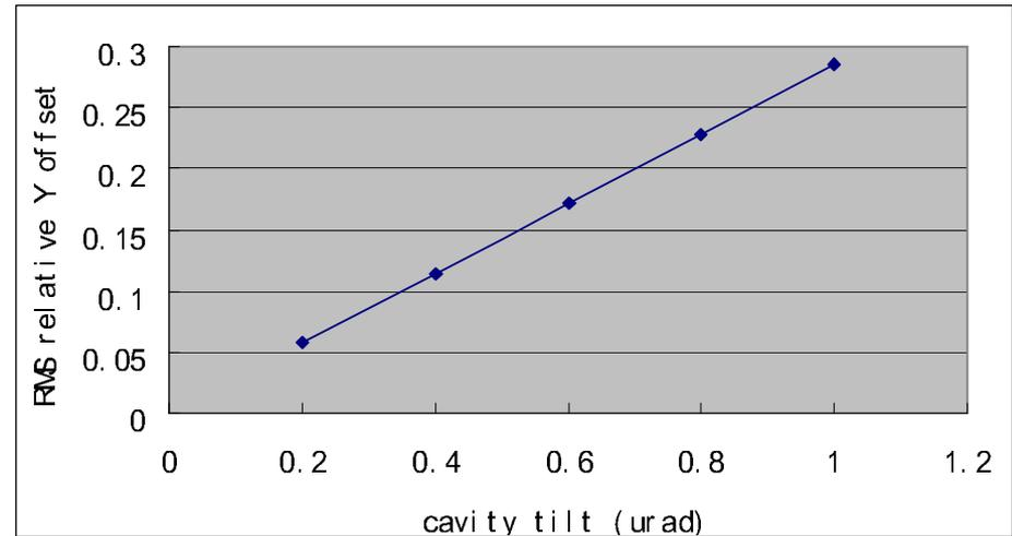
Random cavity tilt jitter tolerance (about 3% luminosity reduction):
