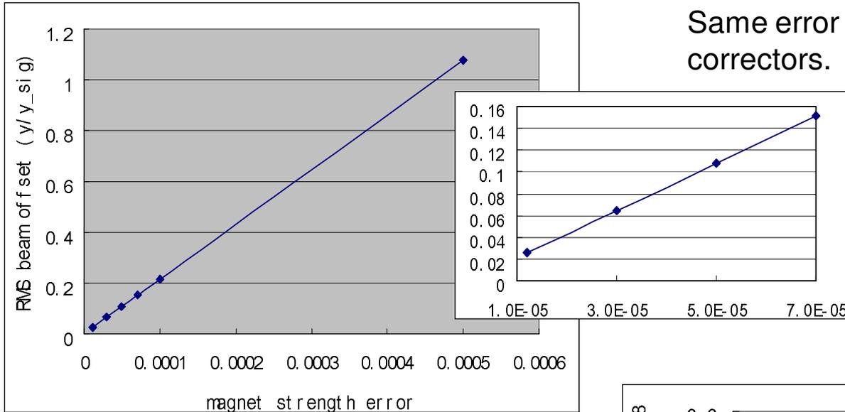
Random magnet strength jitter tolerance (about 3% luminosity reduction):
