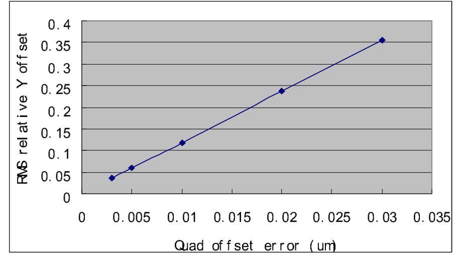
Random quadrupole position jitter tolerance (about 3% luminosity reduction):
