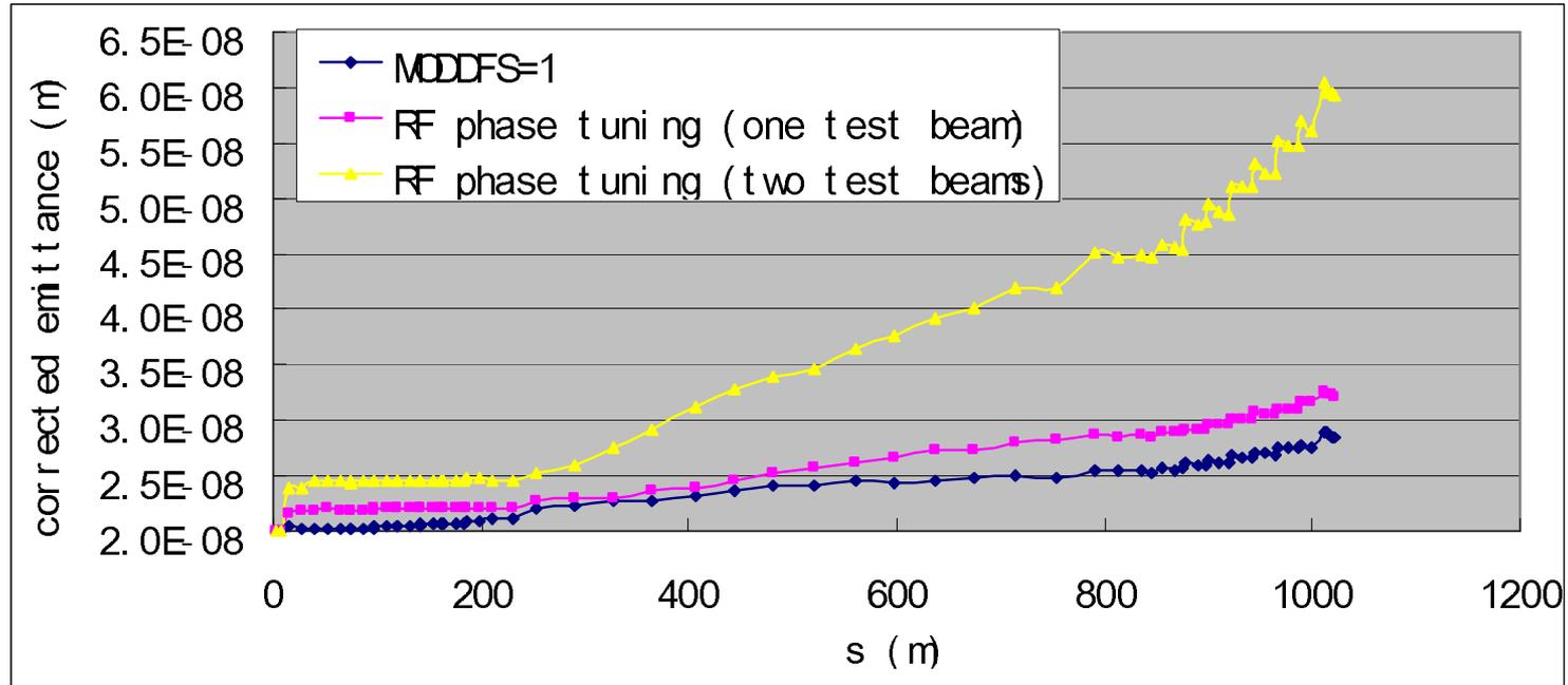
\* MODDFS=1: Both initial beam energy and accelerating gradient are reduced by 10%
