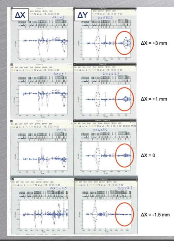
Re-calculated bump based on predicted on-axis fields.
