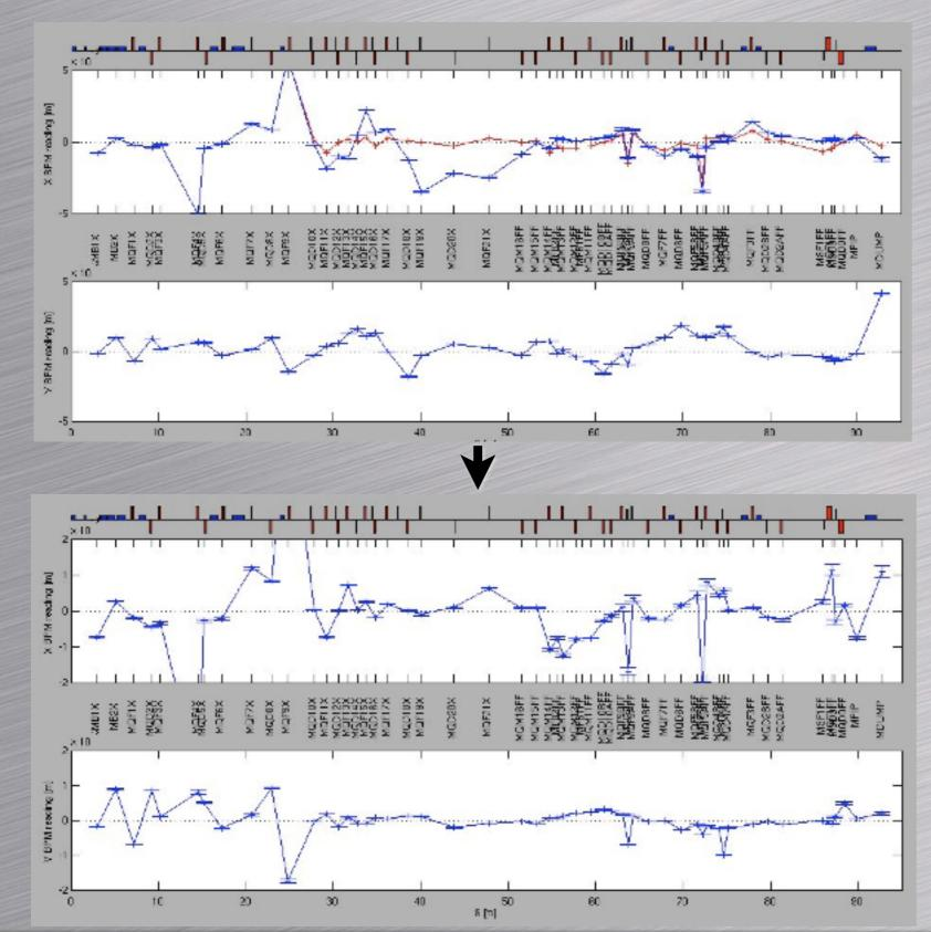
Good Online Model enabled successful auto-correction of orbit for first time (Dec 2009).
