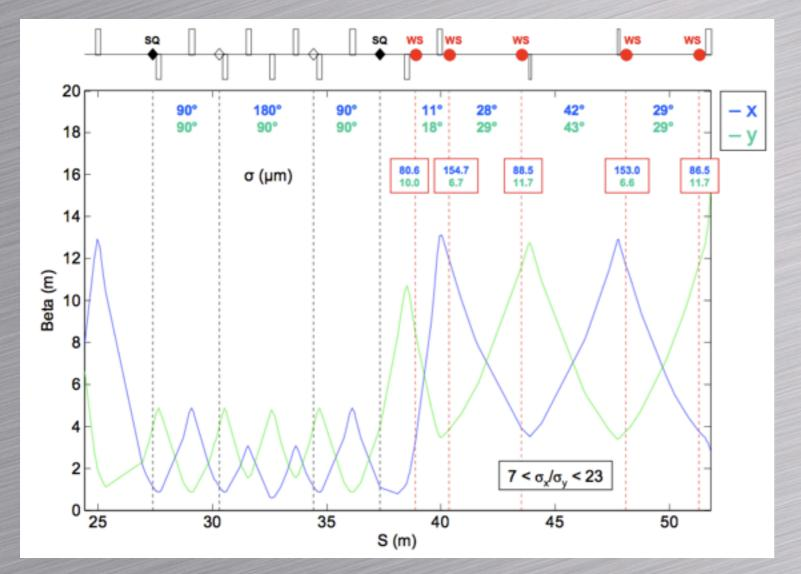
"Reduced correction scheme": \* Scan QK1X/QK3X vs. MW1X y size \* Scan QK2X/QK4X vs. MW3X y size \* Not as good as complete correction (scan QK1-4X vs. vertical emittance), but can be good enough for now and is faster.
