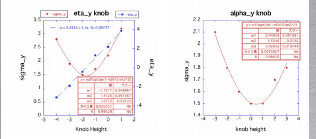
We can minimize the beam size to 1.5um at MW1IP by KEK multi-knob.
