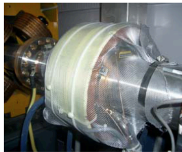
WALL CURRENT & DCCT MONITOR
