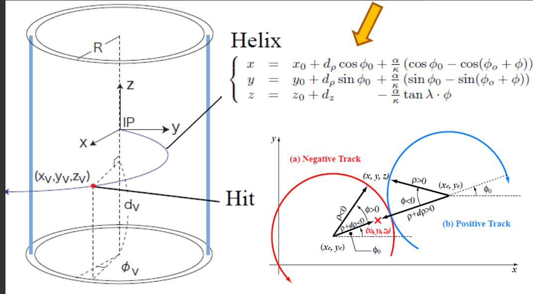
$\left\{ \begin{array}{l} d_\rho: \text{the distance between the helix and the hit in x-y plane} \\ \Phi_0: \text{the azimuthal angle of the hit with respect to the helix center} \\ \kappa: Q/P_t \\ d_z: \text{the distance between the helix and the hit in the z direction} \\ \tan\lambda: \text{the angle of the helix to the x-y plane} \end{array} \right.$
