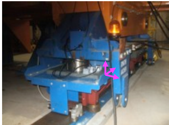
Piston arm is extending Yoke is pushing by the mover.
