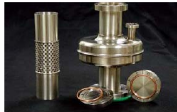
Optimized annular triode pump for experimental areas in the LHC M. Busso and all, LHC Project Report 670
