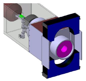
Less dead material Lower gap Better cables paths Stiffer support for tension rods
