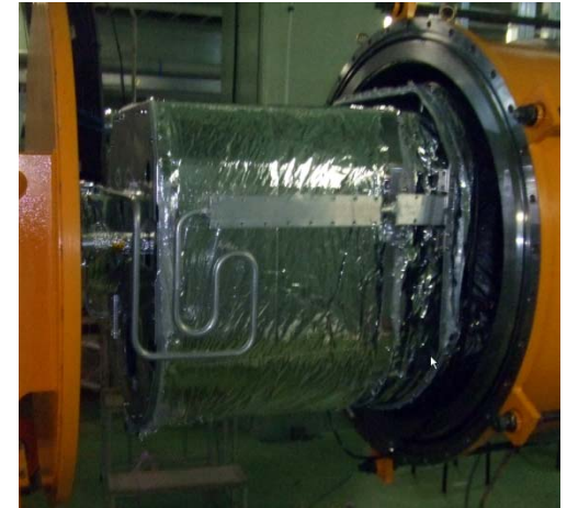
Cryostat ends are covered with the shield plates.
