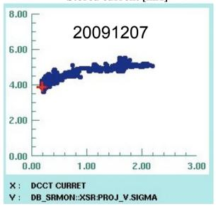
The X-ray SR monitor(XSRM) was affected by the mechanical vibration of the air blower for the RF waveguide. The air blower was located near the grating mirror of the XSRM. The beam profile was smeared and the measured vertical beam size was always larger than 6um. After insert air cushions between the air blower and the ground, the measured vertical beam size was recorded less than 4um, which is not yet limited by the monitor.
