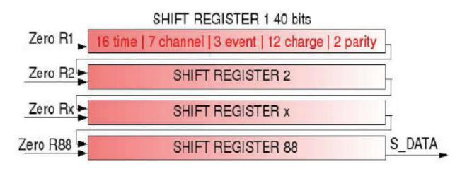
One register per channel with parallel writing and serial readout.
