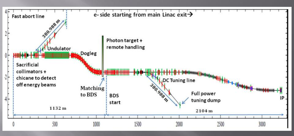
The central integration includes the sources in the same tunnel as the BDS. Relocation of the positron production system to the downstream end of the electron linac means placing it just before the beginning of the electron BDS. These changes need suitable design modifications to the layout of this area. Figure above shows the proposed new layout of the electron BDS
