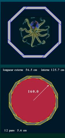
Finding our way between eightfold and dodecagonal Makes 9cm difference for the outer radius Impact on the Hcal, on the end-caps...
