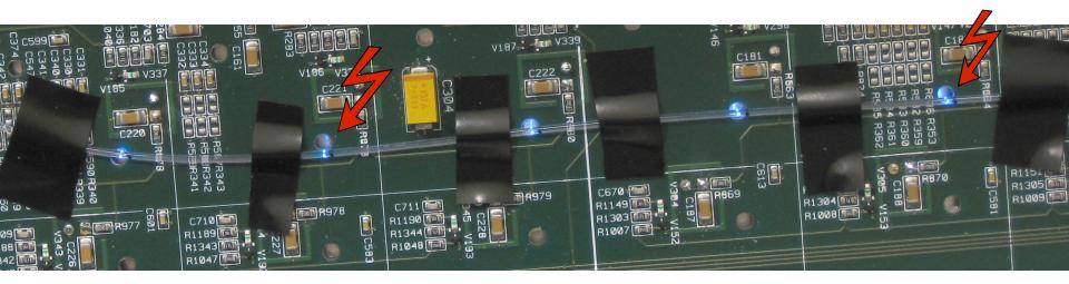
Electrical tape did not fix the bent fiber properly
