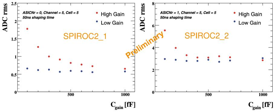
SPIROC2 ADC: 2958 ADC\_chns/V => 2 ADC-counts RMS = 0.68mV Overall characteristic is ok, but much higher noise on ASIC1.
