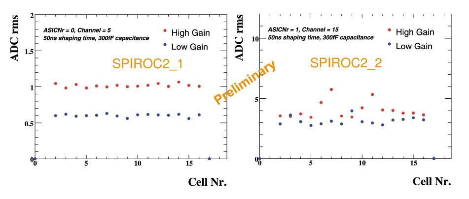
SPIROC2\_2: Higher noise and not equal for the 16 analogue memory cells.
