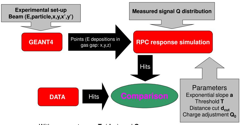
With muons – tune  $\mathbf{a}$ ,  $\mathbf{T}$ ,  $(\mathbf{d_{cut}})$ , and  $\mathbf{Q_0}$  With positrons – tune  $\mathbf{d_{cut}}$  Pions – no additional tuning
