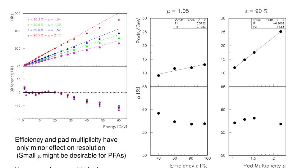
Linear calibration corrections for  $\varepsilon, \mu$  will work (P<sub>1</sub> ~ 0)
