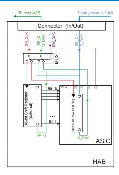
Step 1 : SW\_DAC=1 : Load ASIC DAC SR, 18 x 8 bits per HAB, 864 bits per HBAB for 6 HABs
