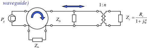
Figure 2: Equivalent circuit of cavity powered through a circulator with the fixed obstacle moving along waveguide
