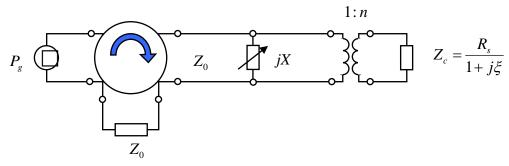
Figure 1: Equivalent circuit of cavity powered through a circulator with the variable obstacle (no moving along wavequide)
