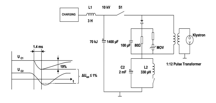
• The linear part of the oscillation of the bouncer circuit is used to compensate the voltage droop caused by the discharge of the main storage capacitor
