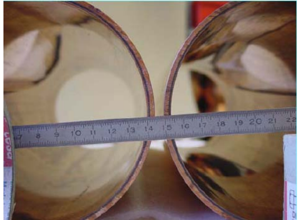
Hot roll bonded Cu-Nb-Cu tube produced at Nippon Steel Co.
