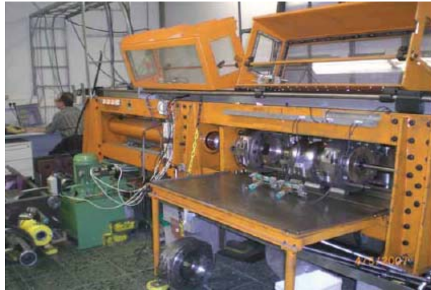
DESY hydroforming machine
