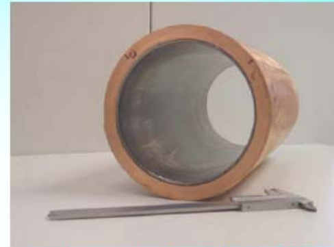
Explosively bonded NbCu tube
