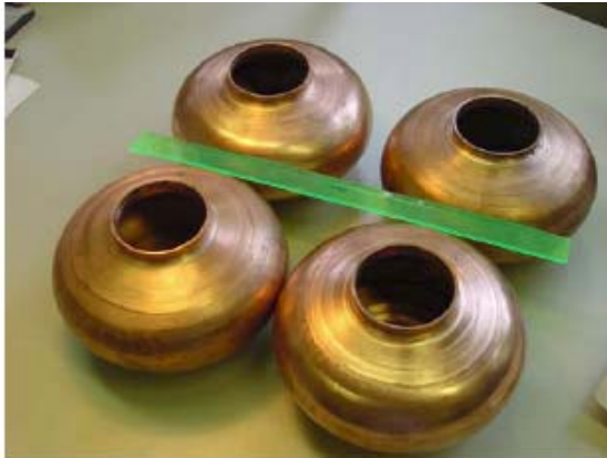
Single-cell Nb/Cu cavities from “sandwiched” tube
