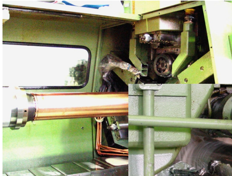
Pot with thick wall by spinning (or deep drawing)
