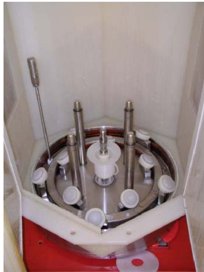
HPR stand inside the clean room at DESY
