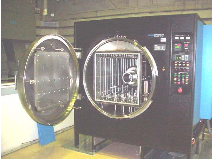
Heat Treatment Furnace at JLab up to 1250 °C, P \leq 10^{-6} Torr
