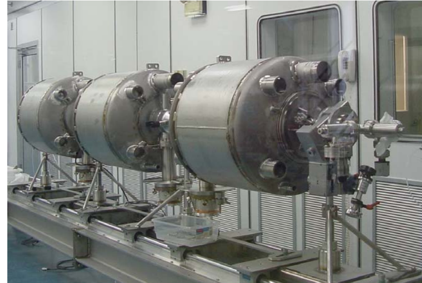
SNS \beta_g=0.61 string at JLab: 3 cavities per string
