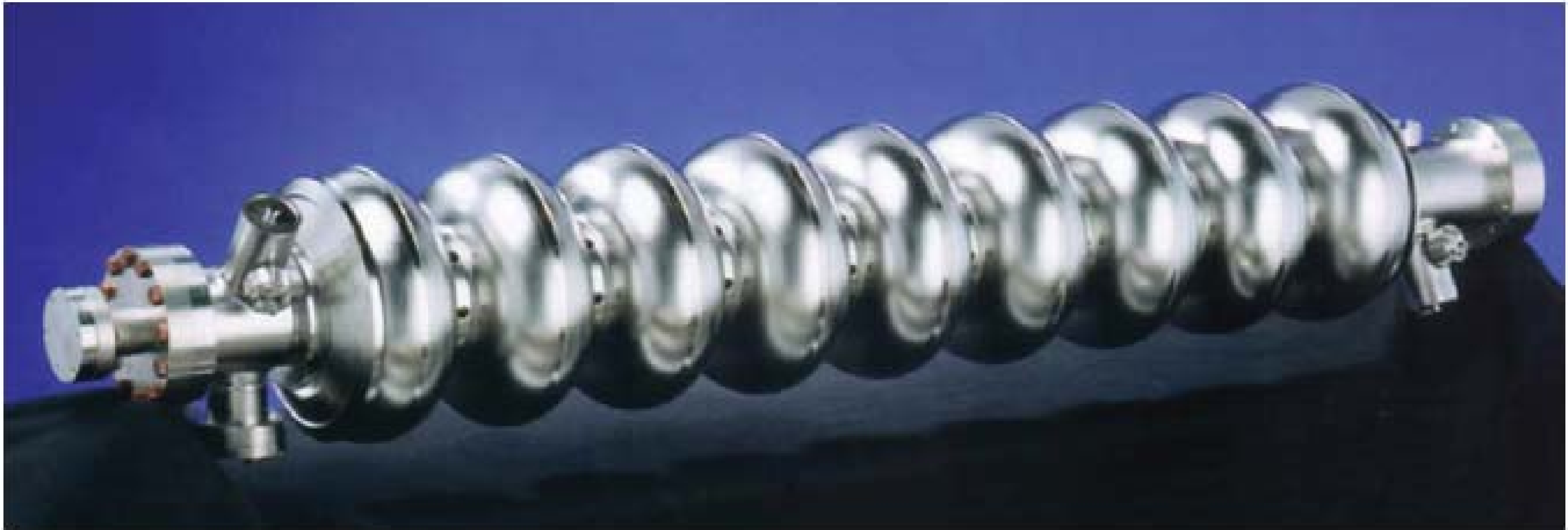
Figure 1.2-1: A TESLA nine-cell 1.3 GHz superconducting niobium cavity.
