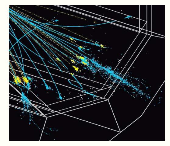
Imaging calorimeter, where spatial resolution becomes as important as energy resolution.
