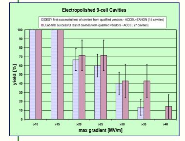
Note: These are results from the vertical CW test at DESY and JLab
