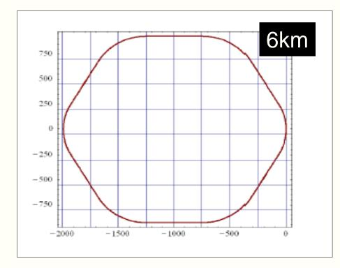
The damping rings have more accelerator physics than the rest of the collider Requires Fast Kicker 5 nsec rise and 30 nsec fall time
