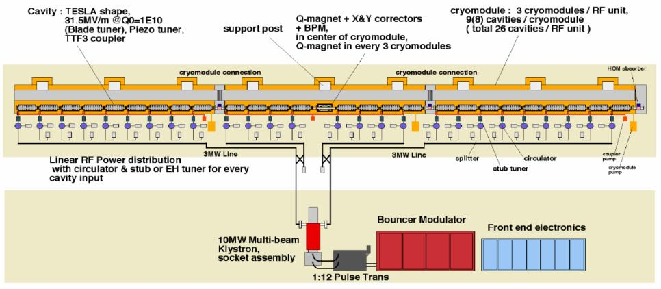
RF power system limits 33MV/m operation.
