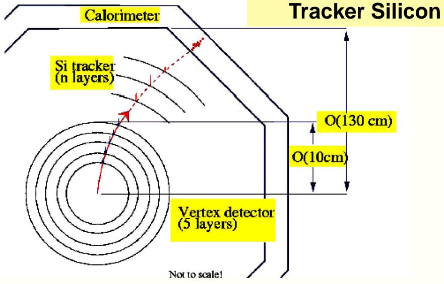
• 5 layers of pixel detectors and 5 layers of Si-strip
