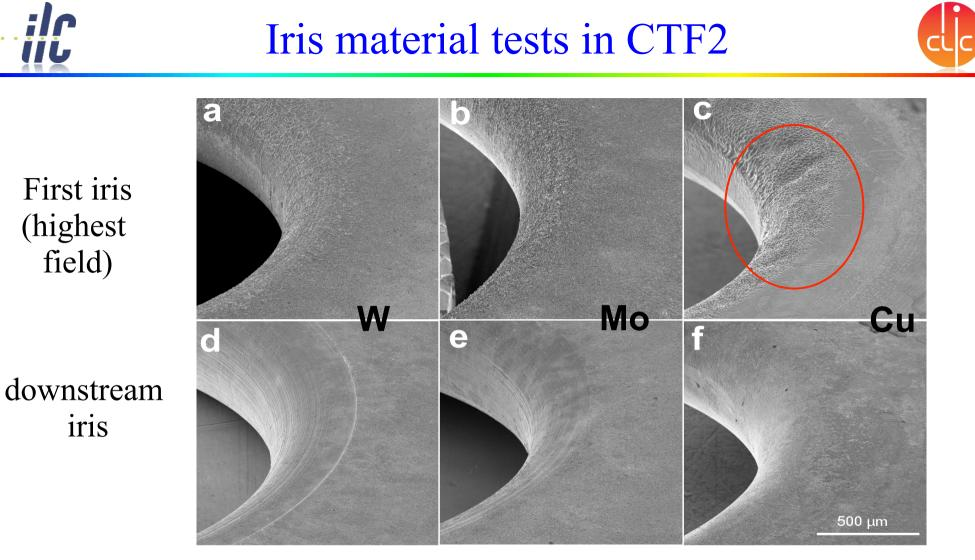
Damage on iris after runs of the 30-cell clamped structures tested in CTFII. First (a, b and c) and generic irises (d, e and f) of W, Mo and Cu structures respectively.
