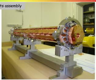
PETS equipped with the power couplers and electronic ruler with pick-up antenna for the phase advance measurements.
