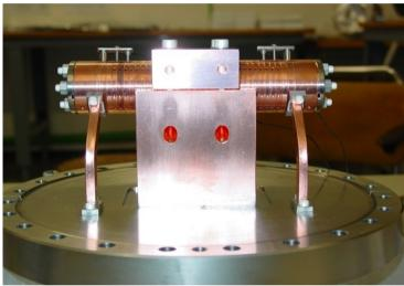
30 cell clamped tungsten-iris structure
