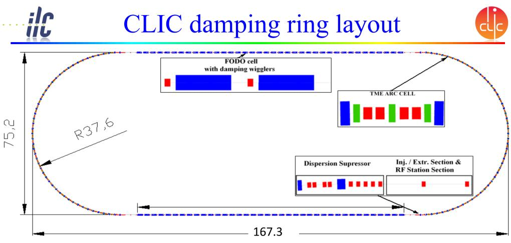
• Total length 421m (much smaller than ILC), beam pulse only 47m
