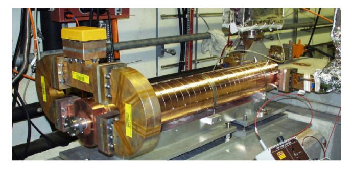
Dipole modes suppressed by slotted iris damping (first dipole's Q factor < 20) and HOM frequency detuning
