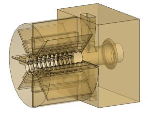
The PETS comprises eight octants separated by the damping slots. Each of the slots is equipped with HOM damping loads. This arrangement follows the need to provide strong damping of the transverse modes.
