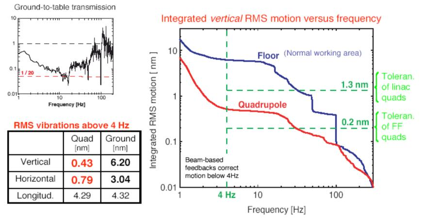
CLIC prototype magnets stabilized to the sub-nanometre level !!
