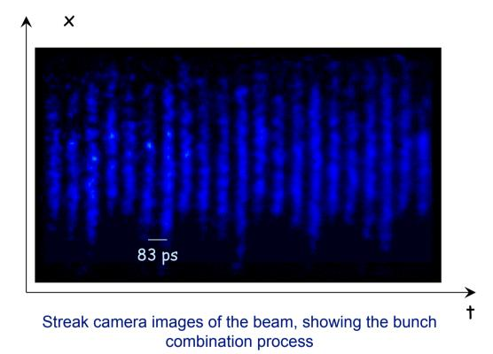
ring combination tost was performed in 2002, at low surrent and short pulses
