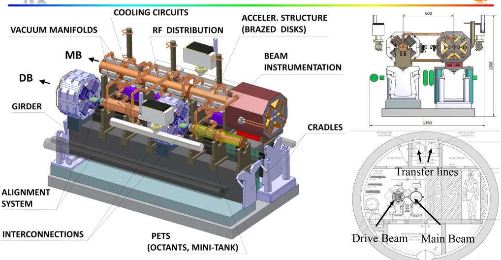
Alignment system, beam instrumentation, cooling integrated in design G.Riddone
