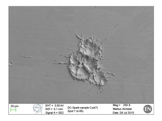
The details vacuum breakdown will be covered extensively in next section. This is one of the two the main effects which limit gradient in accelerating structures.
