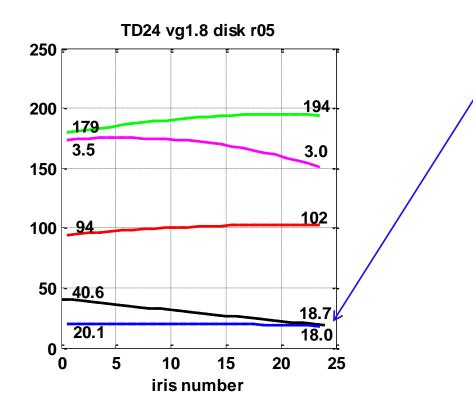
A pulsed surface heating temperature rise of 20 °C corresponds to a compressive stress of 68 MPa.
