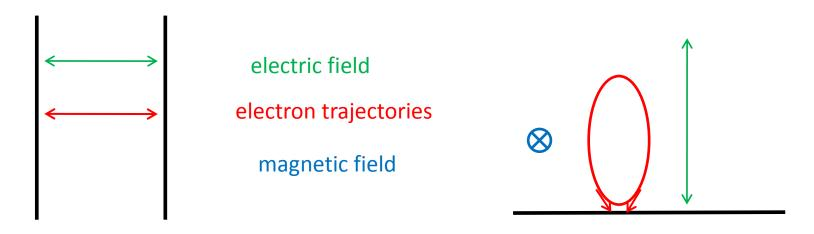
Two- point multipactor, low magnetic field, parallel gap, integer number of rf cycles.
