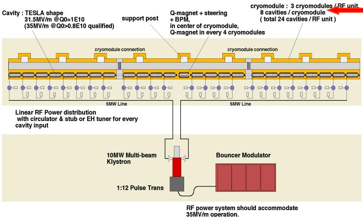
Note: The RF Unit configuration has since been changed from 24 to 26 cavities
