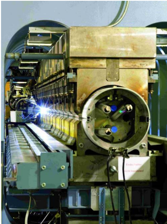
Welding of LHC main dipole cold mass
