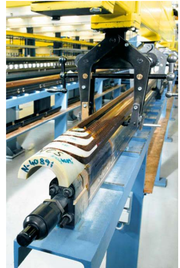
Layerjumps on LHC main dipole winding package
