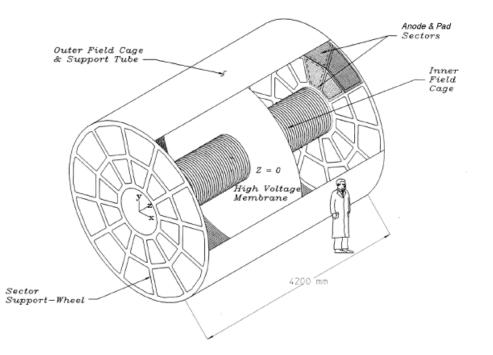
Cathode: 70 µm CLK tensioned to outer support hoop, mounted inside OFC, no mechanical coupling to IFC
