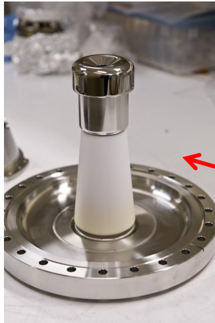
Replace conventional ceramic insulator with "Inverted" insulator: no SF6 and no HV breakdown outside chamber
