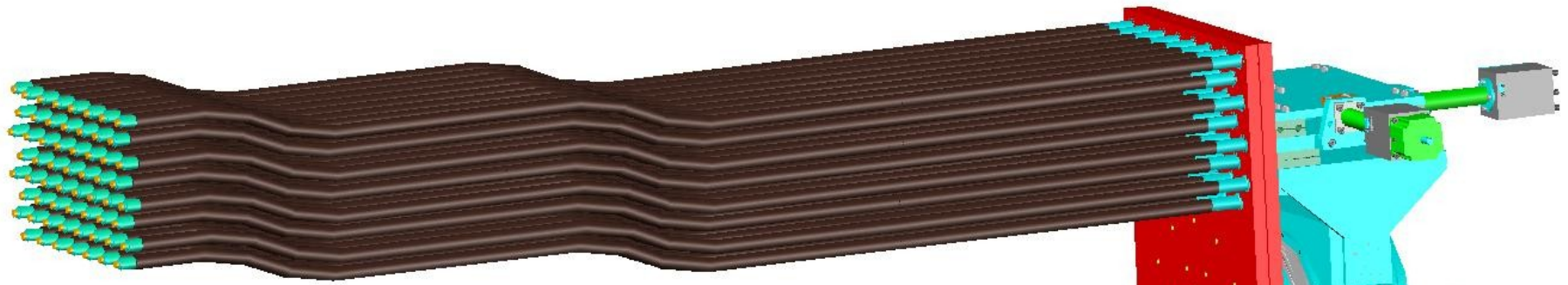
Cables with non organic insulation
