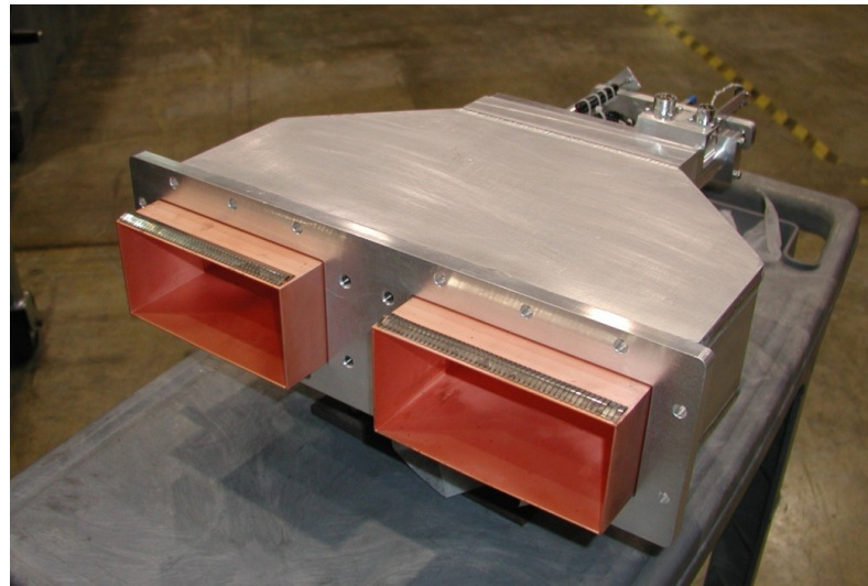
A folded magic-T provides convenient port orientations.
