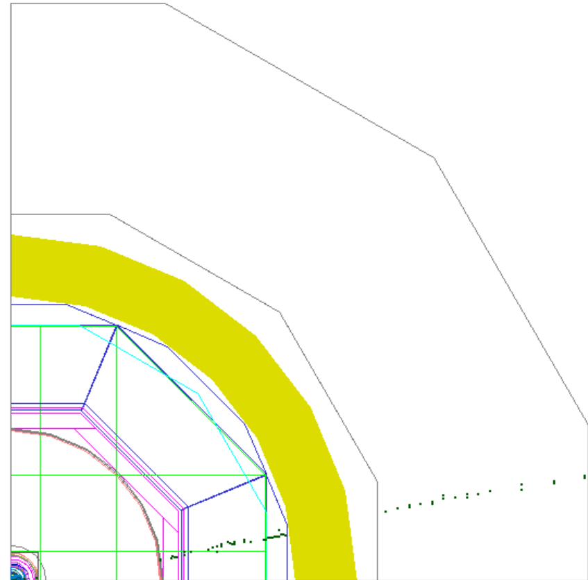
20 GeV muon simulated in the new ILD detector geometry
