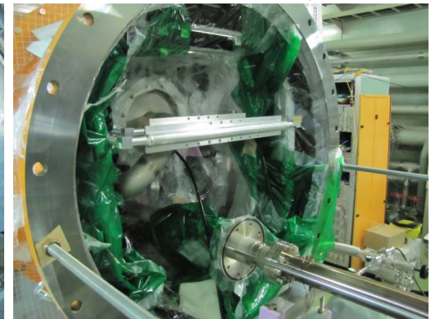
Welding positions were covered with plastic bags.
