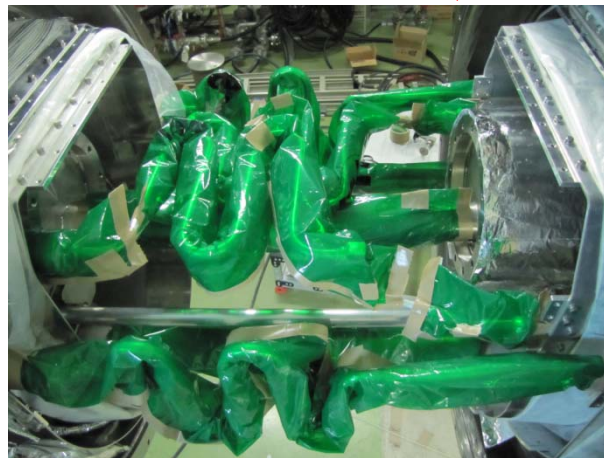
Welding positions were covered with plastic bags.
