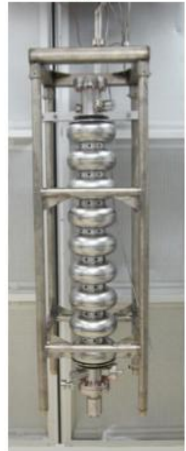
PKU3 is the 3 rd 9-cell cavity built by Peking University SRF Group since 2008
