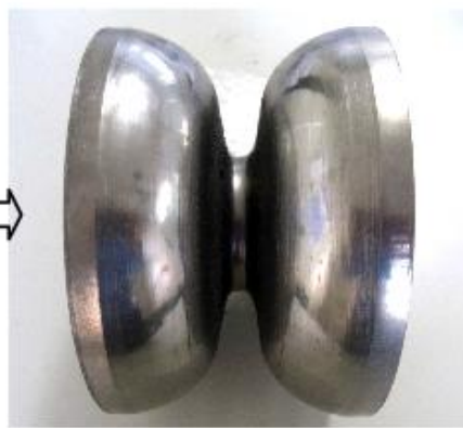
MHI trial of cylinder forming to dumbbell by spinning
