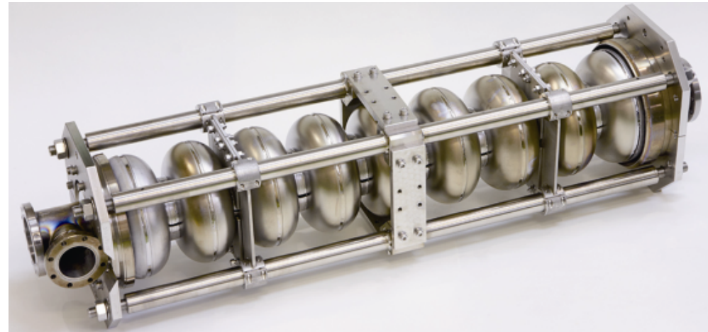
TOSHIBA 9cell Cavity TOS_001 [Without HOM Couplers] 1st. Vertical Test 07/08/2010 Low Current Density EP-II(20 \mu m) with N2 gas, Water flow(1.5hrs), FM_20 2%(50C,2hrs), H.P.R.(10hrs)
