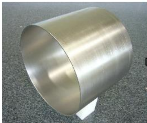
MHI trial of cylinder forming to dumbbell by spinning
