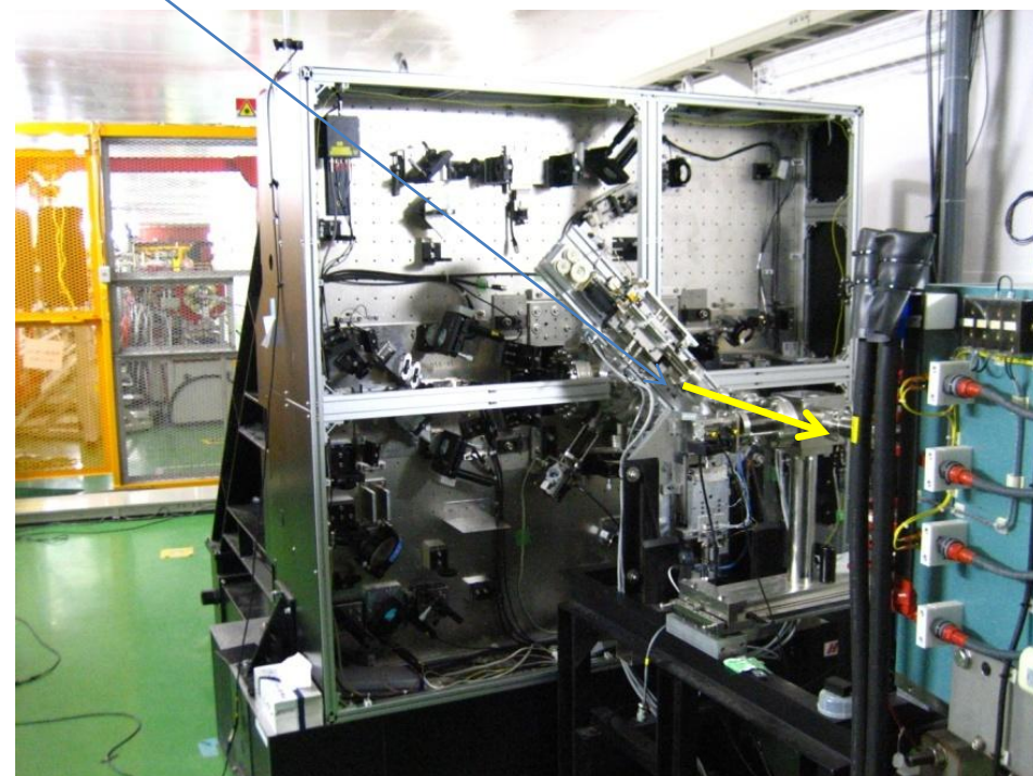
Picture of the vertical optical table installed at ATF2 beam line
