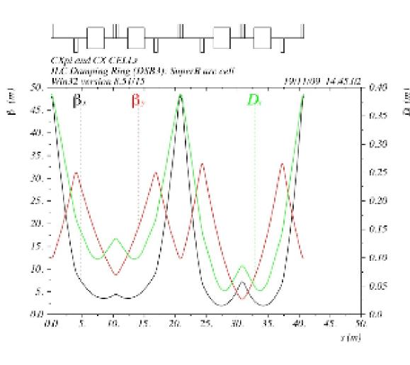
The arc lattice is based on the SuperB arc cells.
