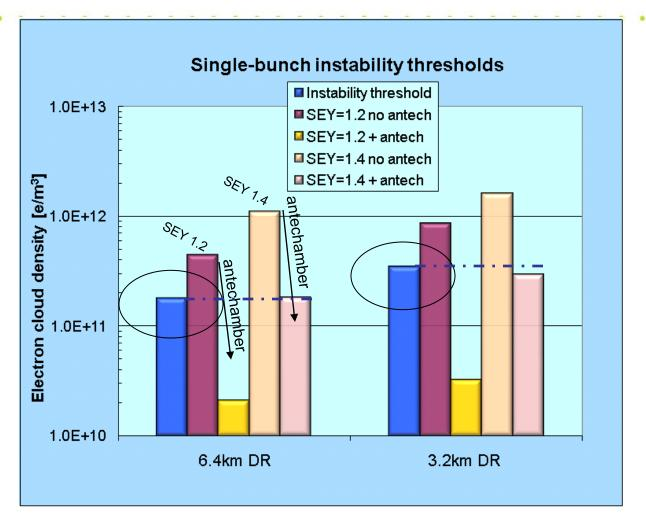
Simulation Campaign 2010: compiled data of build-up simulations compared with the simulated beam instability thresholds. Overall ring average cloud densities are shown for the 6 km and 3 km rings. The surface Secondary Electron Yield (SEY) determines the cloud build-up and density level.
