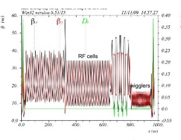
The wiggler straight is located downstream of the RF cavities in order to avoid damage by synchrotron radiation
